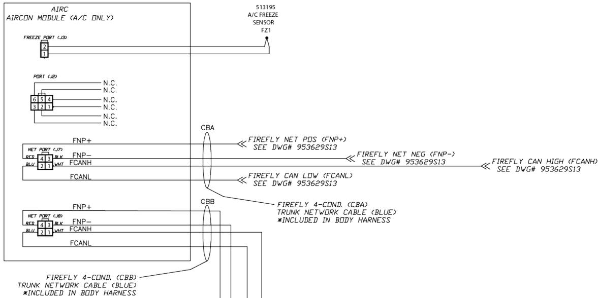
\* SCHEMATIC ONLY SHOWS GENERAL WIRE CONNECTIONS NOT ACTUAL WIRE ROUTING. SEE HARNESS DRAWINGS FOR ROUTING.
