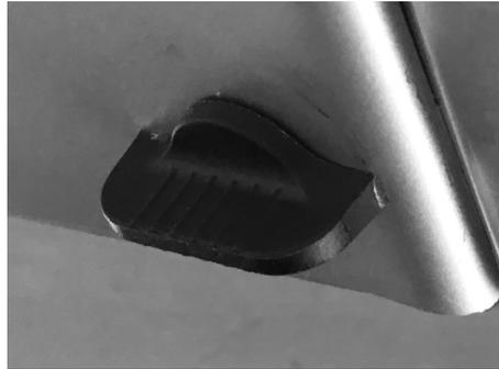
3. Pull straight down to remove cover. Once removed you can store this in one of the rear storage compartments. Reverse these instructions to reinstall.
