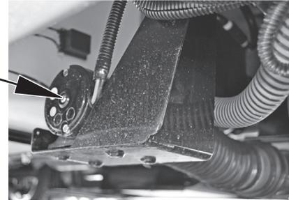
After long periods of non-use, a stuck impeller can be easily broken loose with a screwdriver inserted in the motor shaft slot. Remove the rubber boot, turn the shaft clockwise, and replace the rubber boot.
