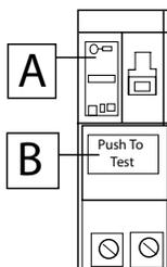
1. With handle A in "ON" position, press PUSH TO TEST button B.
