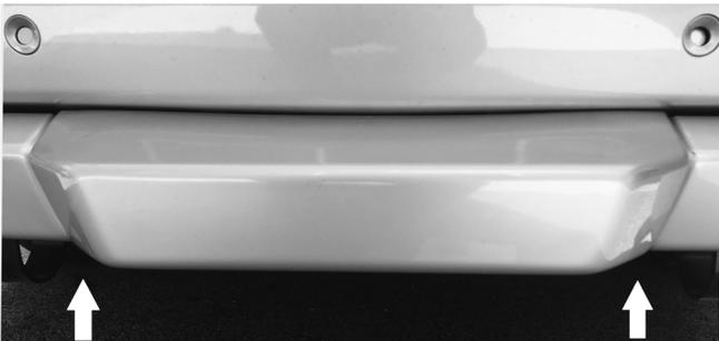
2. Rotate each wing nut 1/4 turn, pull down and remove.
