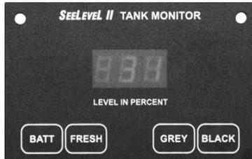
The display is the only system component that is accessed by the user. The display shown above is located in the overhead cabinet behind the the Multiplex Touchscreen. All user input to the display is done using the four buttons along the bottom of the display.
