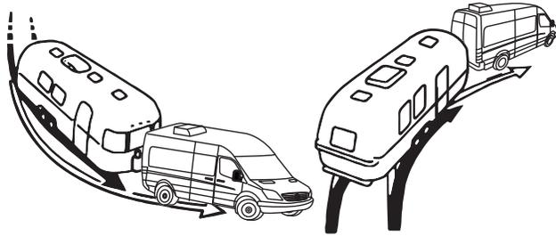
During practice, observe that the tracks made by the trailer wheels are distinctly different from those made by the tow vehicle. Studying this will make it easier for you to correct mistakes. Consider truck- or trailer-type fender or door grip rear view mirrors for maximum visibility. In most states, the law requires them.
