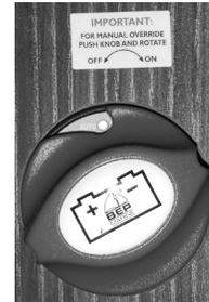
The manual disconnect switch, located at the base of the drivers side rear ottoman behind the decorative access door, is used to turn off power from the battery to the 12-volt distribution panel. Push knob in before manually rotating it to the ON/OFF position.
