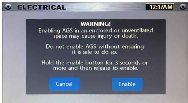
Once enabled, AGS will remain enabled until the Sprinter Ignition is cycled or the generator is manually operated. After the vehicle is started, the AGS will be disabled. You can then return to the cabin to manually re-enable the system. It will then remain active until the vehicle is turned off. Any cycling, on or off, of the vehicle ignition will disable the AGS functionality.
