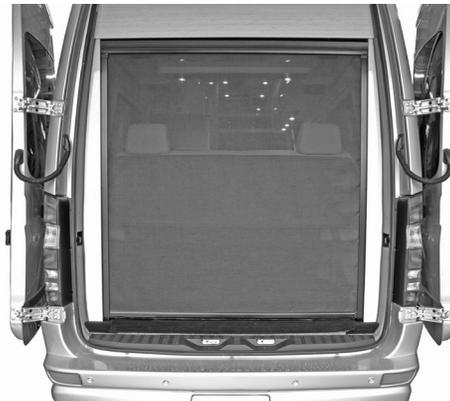
To lower the rear power screen, press the down button on the multiplex control panel once. To stop the power screen in the position that you want, press the button again or allow the screen to stop automatically when it reaches its set limit. To raise the power screen back up press the up button on the multiplex control panel.
