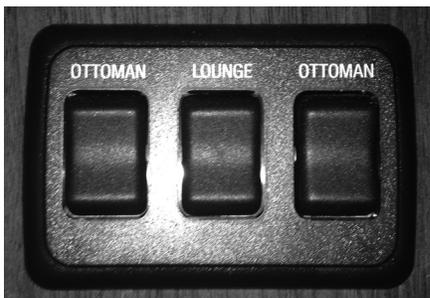
The side ottomans and rear lounge can be converted into a sleeping area by first pulling out the aluminum extension, lowering the pillow extenders, and removing the headrests. Press and hold the switch located under the passenger side overhead storage locker until the lounge flattens completely. This same switch will be located on the driver's side in the Interstate GT model. Lower the powered ottomans on each side of the coach to complete setup.
