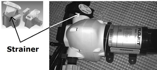
To clean the strainer screen: with the clear plastic at the top, press on the sides of the strainer releasing the tabs holding the clear plastic top in place, hold the sides in, and pull straight up on the clear plastic top to remove the screen assembly. Rinse all debris from the screen. Replace the screen assembly by aligning the screen in the seating grooves and pressing gently down until tabs catch and hold the clear plastic top in place.
