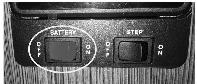
The battery disconnect switch located on the multiplex panel at the entry door is used to separate the 12-volt distribution panel from the converter charging system. When connected to an external AC power source, the 12-volt distribution panel will receive power from the converter and the touring coach will function normally. The batteries will be charged through the converter charging system regardless of if the battery disconnect switch is in the ON/OFF position.
