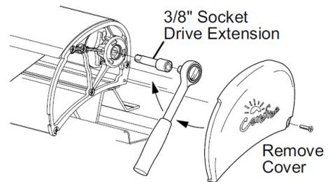
1. Remove thumb screw from backside of decorative awning cap. The cap will be held in place by velcro that must be released before removing.
