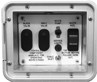
1. Remove the high pressure waste hose by opening the hose reel compartment door and momentarily pressing the “release” switch. Once released the hose can be manually pulled out. Secure the hose at the disposal facility inlet using the threaded or rubber adaptor and open the drip proof valve on the end of the hose.
