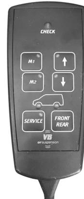
A remote, located on the B-pillar next to the drivers seat, can be used to manually adjust the air suspension. To manually adjust, while parked set the emergency brake. With the engine running, press the up or down arrows to raise or lower the rear of the van. Two memory buttons, labeled M1 and M2, allow for two different memorized height settings. To set, adjust the van to the desired height then press and hold one of the memory buttons.
