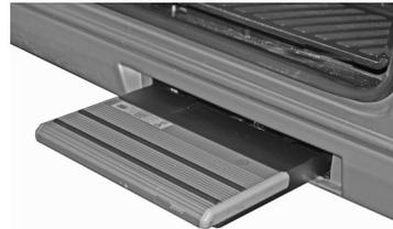
The curbside sliding door has a sliding step with auto retract, step out warning buzzer, and a lock extended switch located on the multiplex panel just inside the sliding door. Please read, understand, and instruct passengers of the following operational and safety information pertaining to the step.
