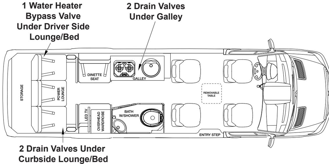
The fresh water system has four fresh water line low point drain valves. There are two under the galley, accessed by removing the drawer below the microwave. Two are located under the lounge, on the curbside, accessed by removing the cup holders. The cup holders lift up and out of the armrest. The water heater bypass valve is located under the lounge on the drivers side.
