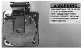
The Power Cord hookup is located on the side of the touring coach. The cord may be stored in the rear exterior compartment. The power cord is plugged into the touring coach receptacle and the City Power Service.
